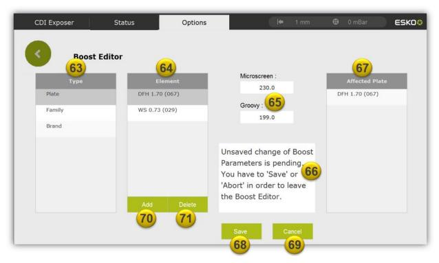
The Pixel Boost values can be assigned to a certain plate type "Plate", a plate family "Family" or to the plate manufacturer "Brand". This must be selected in the "Type" field (63) before changing or adding values.
