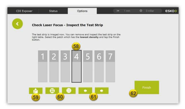
To identify the focus, the plate is taken off the drum (59). The vacuum is switched on and off by using the buttons (60). The fields are measures using a densitometer.
