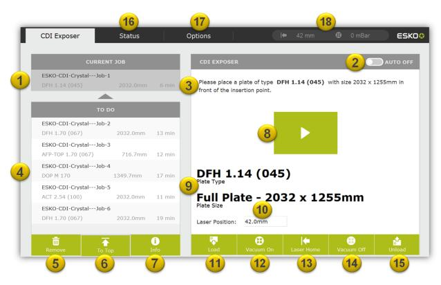
"Current Job" (1) is the current job. Instructions on which plate to install are shown in the "CDI Exposer" (3). The subsequent jobs are listed under "To Do" (4).
