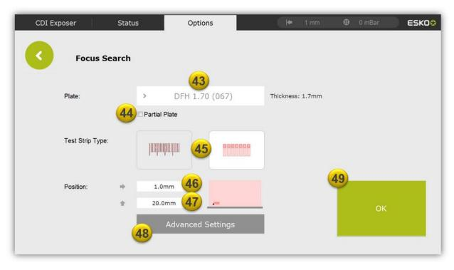
The plate type is shown behind "Plate:" (43). Pushing "Plate" (43) will show the available plate types, from which one is then selected.
