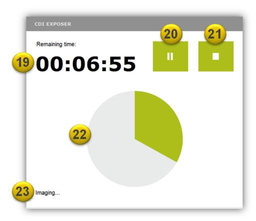
The remaining time (19) is displayed, along with a graphical representation of the progress (22). The exposure can be paused with 20 or stopped with 21. The executed action (23) is displayed at the bottom left, e.g. load - expose or unload.
